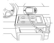
**Note:** When you choose a mounting area for the controller, make sure it is close enough to the Audio Adapter's mounting area so the controller's cord will reach the Audio Adapter. The controller's cord is about 5 feet (152 cm) long.
